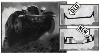
"FLOATING-CUSHION" WHEELS-the final step com-pleting the levelized, vibrationless ride. Inde-pendent front-wheel suspension makes smooth riding no matter how rough the road. When one front wheel strikes a bump or rut, the wheel -independently of the rest of the car-rises and falls with the bump. The shock is absorbed by
