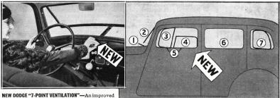
NEW DUDGE "1-FUNI VEHILATION"—An improved and perfected ventilating system. (1) Coul ven-tilator. (2) Windshield opens or closes by means of crank on the instrument board. (3) Front half of forward window may be swung open in "butterfly" fashion. (4) Rear half of the window can be raised or lowered independently of the "butterfly". (5) Both halves of the forward window may be locked into a single unit and raised or lowered together, just as with a regular window. (6) Rear door window,
